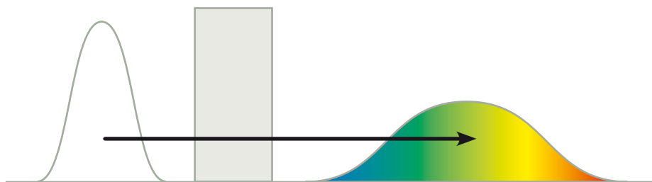
Figure 1: Broadening of a pulse by propagation through an optical medium (schematic drawing)
